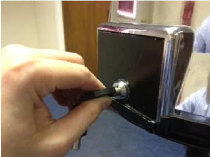
1. Undo then remove cash lock using the correct key.
