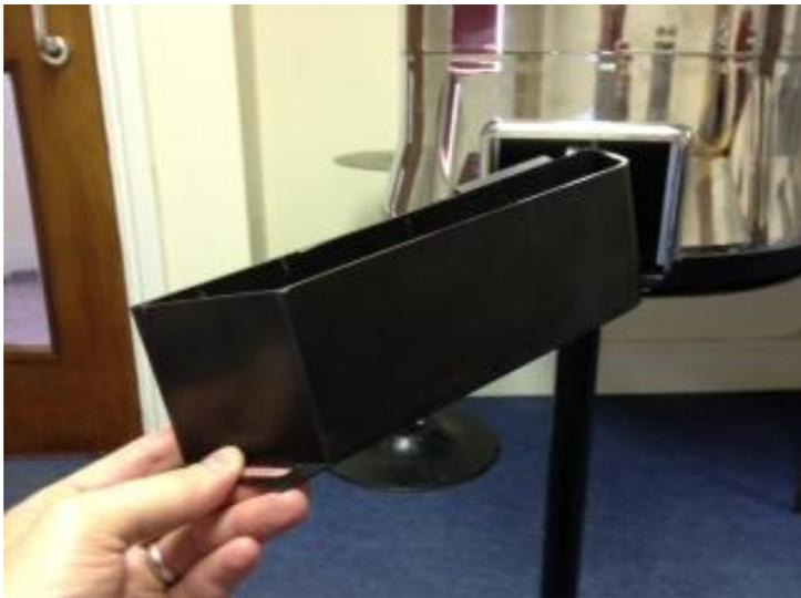
3. Remove the silver locking bar and remove the plastic coin draw
