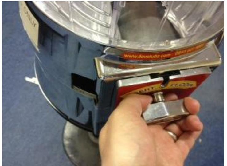
16. Test handle to make sure the coin mech is in place properly and it is turn the barrel.
