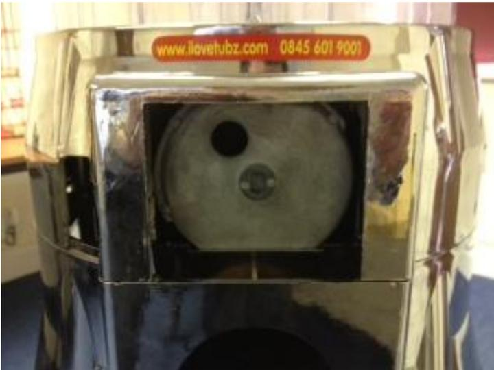
9. To replace coin mech make sure the barrel is positioned with the hole at 11 o'clock
